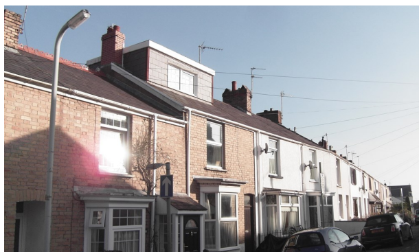
Extensions and alterations at roof level change the line and rhythm of terrace skylines to the detriment of the host building and wider terrace
